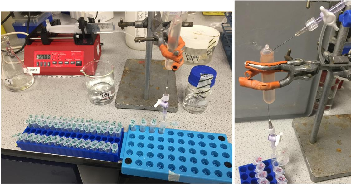
Figure 4.4: Gradient fractionation setup. This method is used to recover DNA from the ultracentrifuge tubes. NE-1000 Programmable Single Syringe Pump was used to retrieve equal volumes of density gradient fractions from ultracentrifuge tubes. For each sample tube, 50 sterile 2-mL microcentrifuge tubes labelled with sample and fraction number (1–50; heavy to light) were prepared. The pump rate was set to retrieve about 5 drops per tube (ca 125  $\mu\text{L}$ ).
