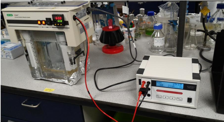
Figure 3.5: DGGE setup with the gel attached to the core assembly immersed in ca 7 L  $1 \times$  TAE buffer
