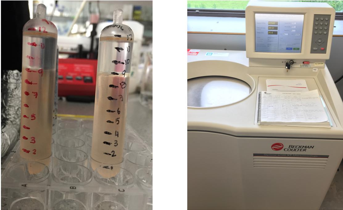
Figure 3.4: Left: Ultracentrifugation tubes comprising cesium chloride stock solution, enriched DNA and *E. coli* internal standard. Right: Beckman Coulter ultracentrifugation machine used in this study
